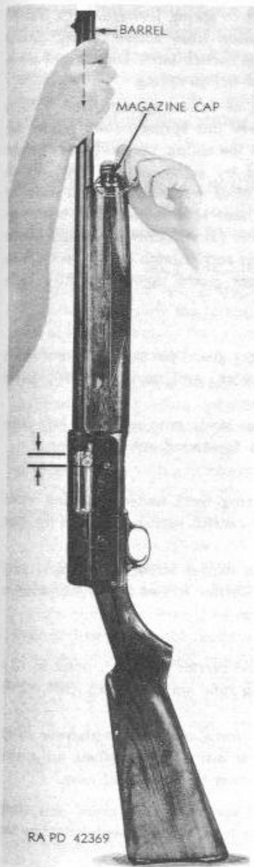
Figure 124—Holding Barrel—Slightly Retracted While Removing Magazine Cap—Savage Shotgun, M720
